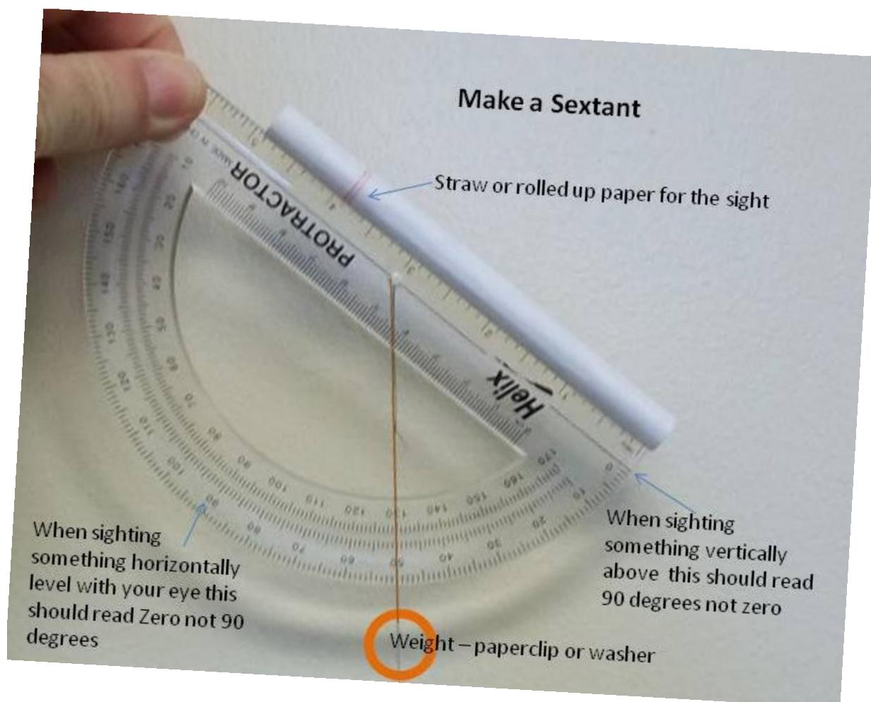
The string tells us that this sextant or protractor is being held at 40 degrees from the horizontal. (Remember to switch the markings or it will read 50 degrees like the one in this picture!)
